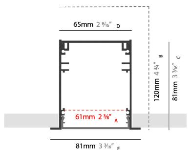
A: OPENING WIDTH B: RECESS DEPTH C: PROFILE HEIGHT
